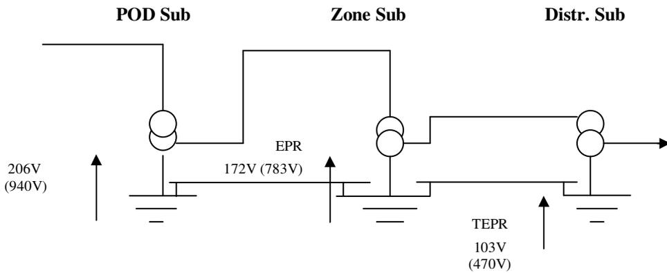
**33kV Fault: New EPR & TEPR values vs original EPR values**
