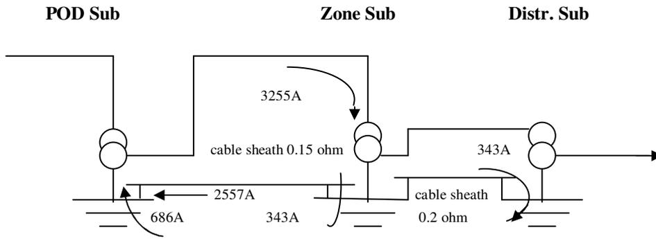
**33kV Fault: Fault currents re-calculated with cable sheath bonding included**
