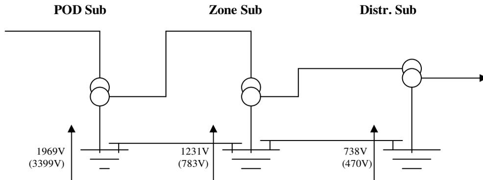
**Maximum EPR values AFTER cable sheath bond is added between Zone and Distribution substations**
