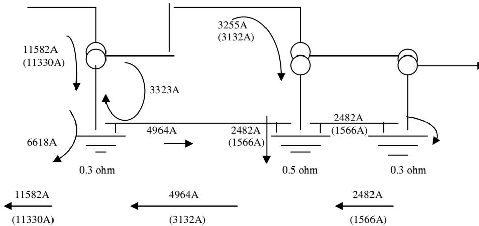
**Maximum fault current values AFTER cable sheath bond is added between POD and Zone substations**
